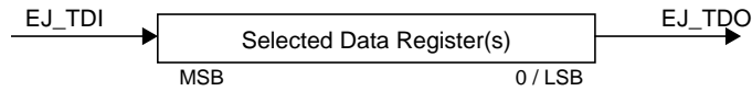
Figure 5-4 EJ_TDI to EJ_TDO Path for Selected Data Register(s) when in Shift-DR State
