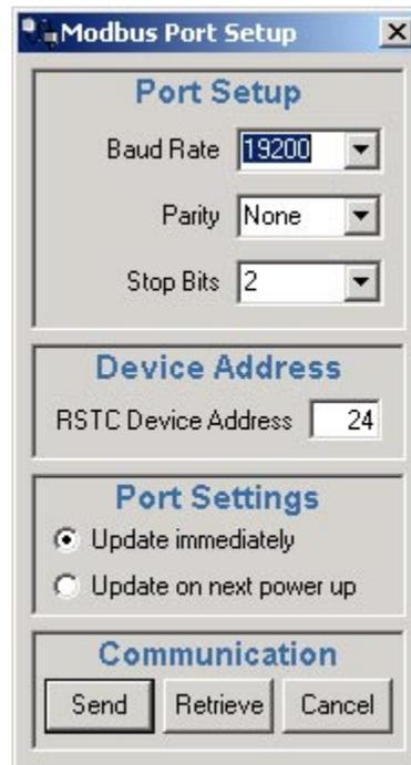
Figure 24 MODBUS Port Setup Screen
