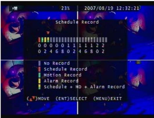
Within a 24 hour period, the user can adjust each channel's frame rate by record mode such as schedule, motion detection, and alarm record. Press the
