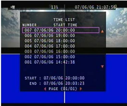
**Time List:** Selecting Time List displays a list of continuous or scheduled recordings separated in one hour segments. Select a recording using the mouse or arrow keys and click/press enter to playback the corresponding recording.
