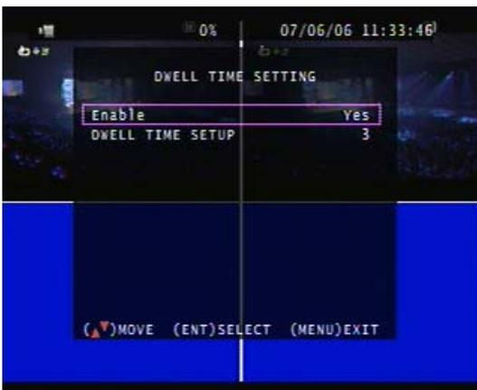
Dwell time is the number of seconds each camera image remains on the screen before switching to the next when the DVR is in single camera mode and Dwell Time is enabled.
