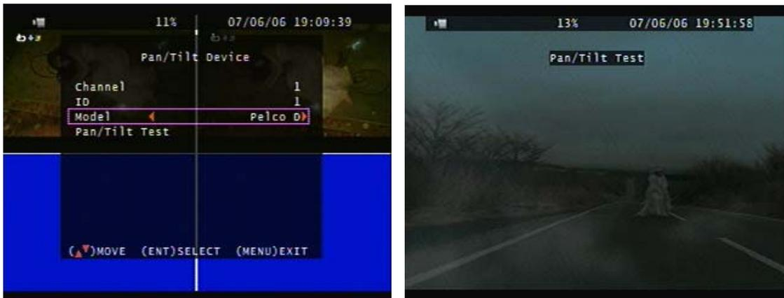
From the Pan/Tilt Device setup screen, the channel, ID and Model of PTZ can be setup. PTZ cameras can be controlled using a combination of the front buttons and the mouse:
