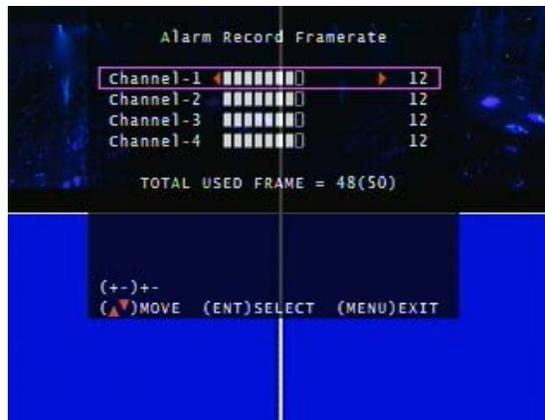
\*Each channel has its own frame rate adjustment for each recording mode.
