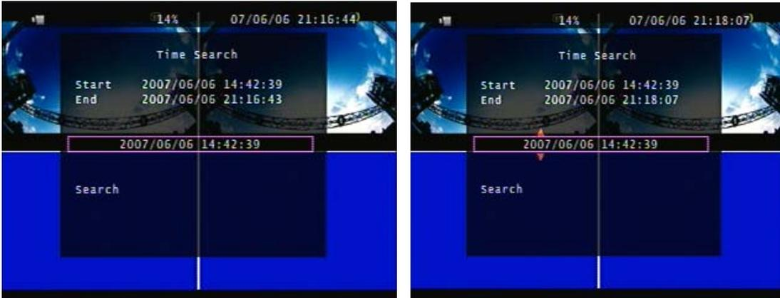
After the required date and time have been entered, move the selection to the Search button (bottom left of the screen) and then press ENTER/Click to start playback.
