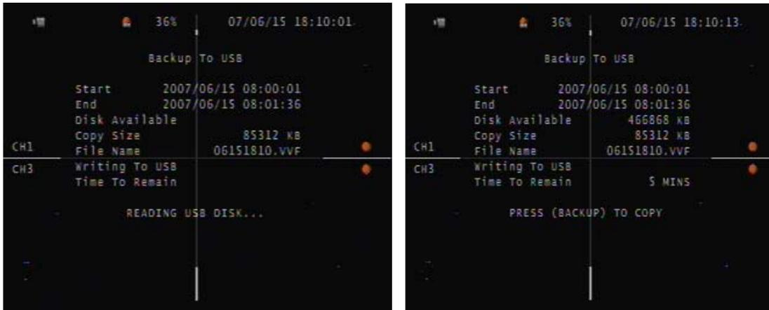
3) After the “Reading USB Disk” message disappears, the backup information will be displayed on screen and the user now can press the Backup button to start the file backup process. When the backup is complete, press the menu button to exit the USB backup screen and return to live video mode.
