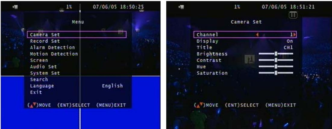
Select Camera Set from the Main Menu. Select the appropriate Channel (camera) and adjust the properties to provide the best video picture.
