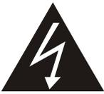
The lightning flash with arrowhead symbol within an equilateral triangle, is intended to alert the user that insulated dangerous Voltage is contained within the product's enclosure. This may be of sufficient magnitude to constitute risk of electrical shock to persons opening the enclosure.
