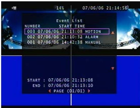
**Event List:** Selecting Event List displays a list of recordings by both time segment and type of event – Motion, Alarm or Manual. Select a recording using the mouse or arrow keys and click/press enter to playback the corresponding recording.
