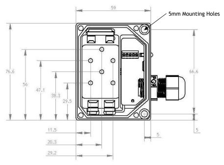
The T24-ACMi has two mounting holes as shown above; these mounting holes are external to the seal but still covered by the case lid to offer fixings for some environmental protection. In addition mountings can be made through the back of the case however a seal or gasket must be used to maintain environmental protection.
