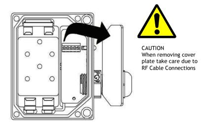
The input connections are accessed by lifting the right hand cover plate, this plate incorporates the T24-ACMi Antenna; take extra care when re-assembling that the grey UHF cable is attached to the antenna socket.
