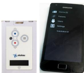
The caregiver devices are portable and wireless sensors that accompany professionals and notify, through sound and light, about the existing alarms. They have a screen display that identifies the customer, the type of alarm and the location where it happened. They can also be used to resolve or silence active alarms.
