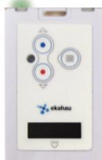
In a normal state of the device, within network coverage, with battery and no active alarm, it presents a flashing green light.
