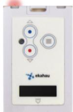
If a caregiver device is not under wireless coverage, the left light flashes with red colour. And Out-of-range alarm will appear in web application (It is considered a system alarm).
