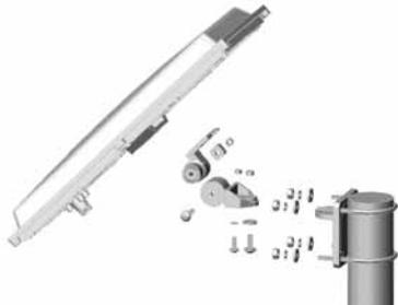
Satellite antenna and mounting adapter
