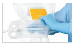
▶ Bend your fingers and pull so that the rail opens. The rail should open easily. The port of the connected Sartoclear Dynamics® DE Bag and the Magmix Bag is now opened.
