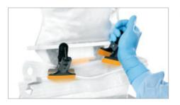
▶ Use the four Clamps for Powder Transfer (B4) to keep the plastic film in position and to protect the rails during powder transfer. Gently push the clamps in the corners for the best protection.
