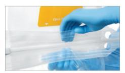
▶ Bring four fingers behind the plastic lip on the Sartoclear Dynamics® DE Bag below the text "Open here" on the yellow folding plate. Bring your other hand behind the lip on the Powder Transfer Adapter.
