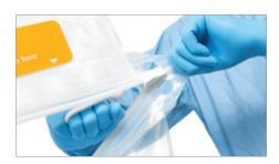
► Hold the two ends of the rails together and pull the Zipper. The Sartoclear Dynamics® DE Bag and the Powder Transfer Adapter are now connected.
