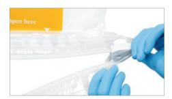
► Insert the rails of the Powder Transfer Adapter in the other inlet of the Zipper so that the rails of the Sartoclear Dynamics® DE Bag and the Powder Transfer Adapter seal together.
