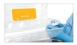
► Take the Zipper **(B3)** and insert the rails of the Sartoclear Dynamics® DE Bag in the Zipper. Around 1 cm of the rails should come out. (See also 3d-print on the Zipper for a correct insertion of the rails).
