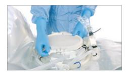
▶ Remove the 8" white plastic cap from the Magmix Bag by loosening the tri-clamp
