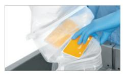
▶ Push the yellow folding plates inwards so that the plastic film completely covers the rails to prevent that DE will stick to the rails.
