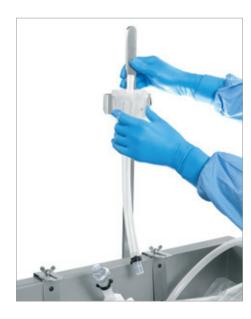
► Open the quick connector on the Magmix Bag and connect the Filterline. Take care that the vent filter does not get in contact with the liquid.
