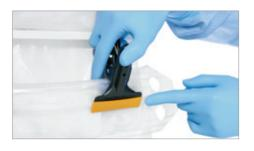
► The yellow silicone lips should go over the rails on the outside of the Powder Transfer Adapter.
