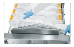
▶ Place the OUTLET plate at the other end of the holder in such a way that the text "THIS SIDE UP" is visible from above.
