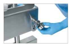
► For Sartoclear® Pilot Filter holder the positioning bars have to be removed for an easier off-loading of heavier filtration devices.
