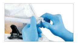
➤ As soon as the Clamps for powder transfer are positioned correctly the plastic bar can be opened to release the powder.
