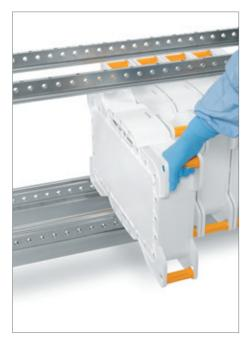
▶ Pull the filter out of the holder until the second groove reaches the first rail.
