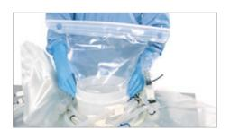
▶ Put the Powder Transfer Adapter (B2) on the gasket
