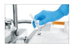
▶ Place the INLET plate of the manifold set at one end of the holder in such a way that the text "THIS SIDE UP" is visible from above.
