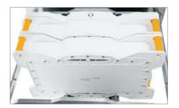
▶ Place the required amount of Sartoclear Dynamics® Filters between the INLET and the OUTLET plate. The text "THIS SIDE UP" and the Order and Lot# should be visible from above.
