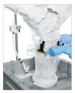
▶ Gently shake the DE Bag up and down to speed up the transfer of DE
