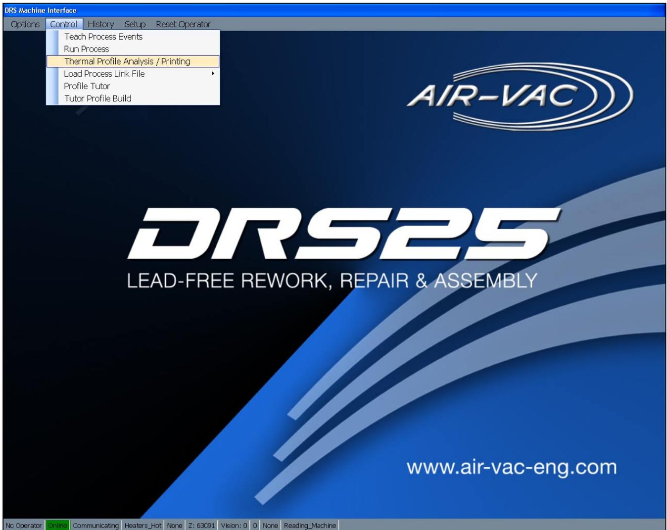
After a new thermal profile is created, the Thermal Profile Analysis tool is used to analyze the profile.
