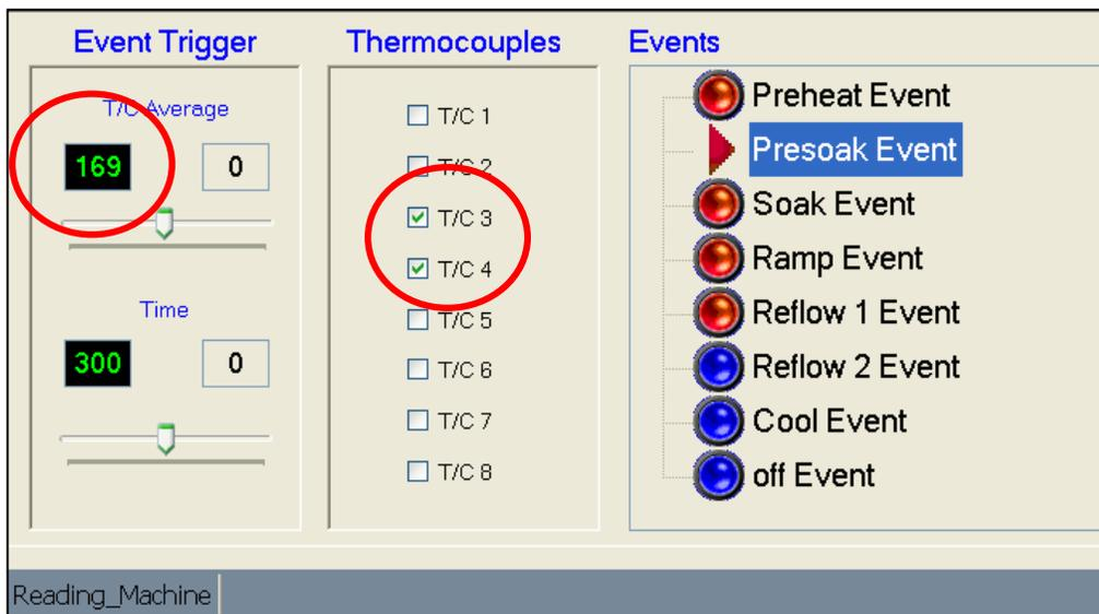
The **Soak Event** will continue until T/C#3 and #4 (average) reaches 200°C (Lead-Free profile). Time in Soak stage is automatically recorded.
