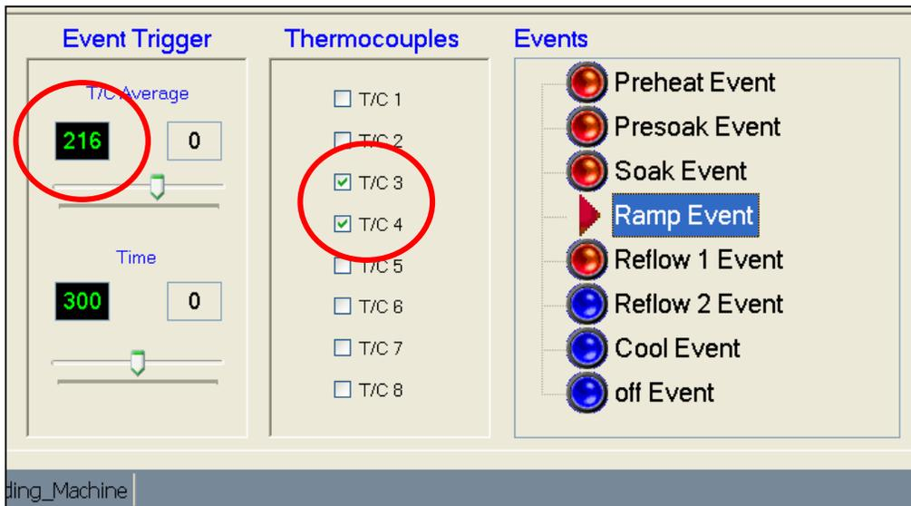
The **Reflow 1 Event** will continue until T/C#3 and #4 (average) reaches 235°C (Lead-Free profile). Time in Reflow 1 stage is automatically recorded.
