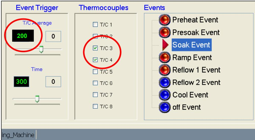
The **Ramp Event** will continue until T/C#3 and #4 (average) reaches 216°C (Lead-Free profile). Time in Ramp stage is automatically recorded.
