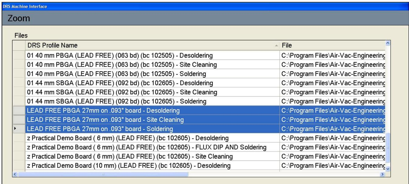
1. Double click on the Desoldering profile to open it.
