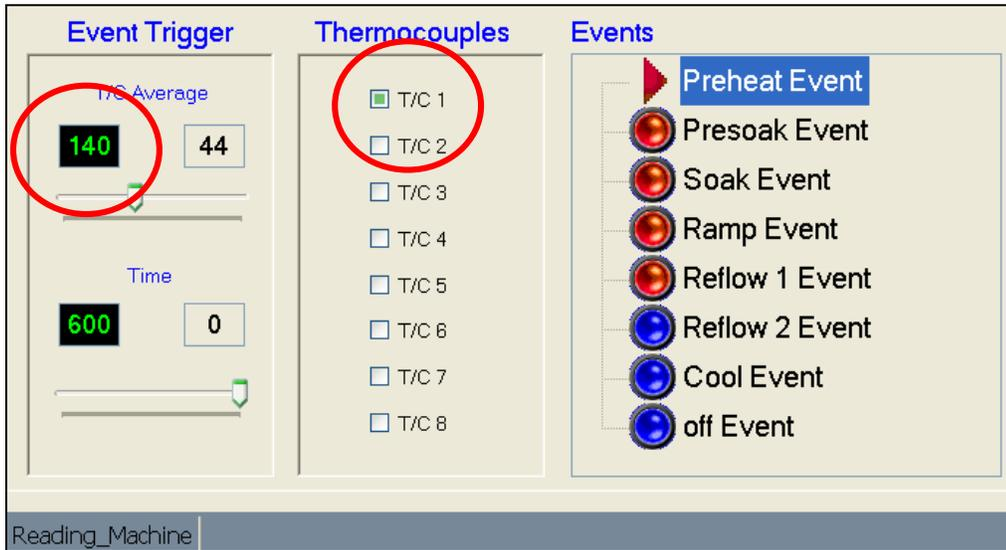
The **Presoak Event** will continue until T/C#3 and #4 (average) reaches 169°C (Lead-Free profile). Time in Presoak stage is automatically recorded.
