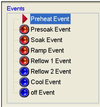
All master profiles typically have seven (7) stages (Events): Preheat, Presoak, Soak, Ramp, Reflow 1, Reflow 2, and Cool.
