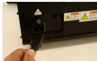
Fig. III-F-3. Connect power cord to left side of instrument
