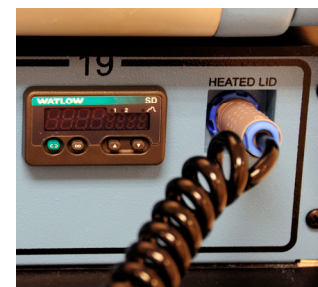
Fig. IV-B-1 Heated Lid connection.
