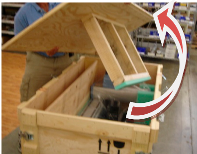
Fig. III-A-1 Unlatch and remove crate lid.
