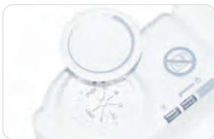
Improved economy may be achieved by limiting the thermostat rotational range, by means of the mechanical 'peg and hole' feature hidden beneath a removable cap on the thermostat knob.
