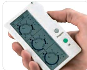
The MB programmer communicates with the heaters and controls a comfort or setback thermostat as per the times set in the programmer.
