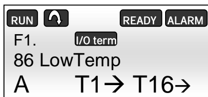
Figure 5.1-3, Low temperature alarm on the NXP panel
