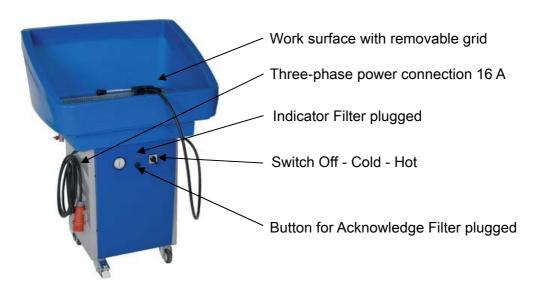
Fill cold, clean water or the suitable cleaning agent in until its level is about 3 cm below the grid (55 l) in the tank and the cleaning tub.
