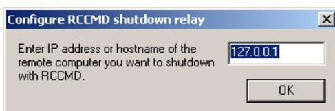
Configuration of the RCCMD relay: This turns the RCCMD Client into a RCCMD Server that can shutdown several 100 RCCMD Clients simultaneously – much faster than a CS121 at the same task.
