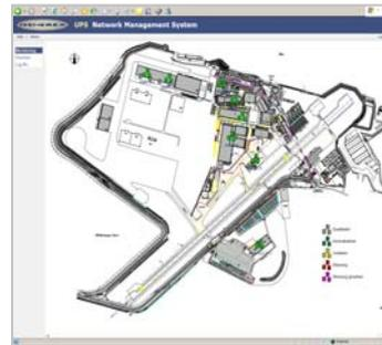
UNMS II at the AIRBUS location in Hamburg for monitoring many UPS devices for the A 318, 319 and parts of the A 380 production facilities.
