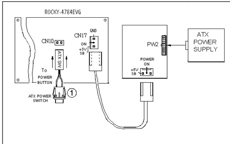
Connect the ATX power button switch to the CN10 (power button) and connect the power cable from Backplane to CN17 of CPU card.
