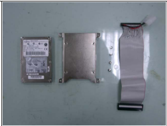
Fig. 2-19 A 2.5" HDD and the HDD bracket
