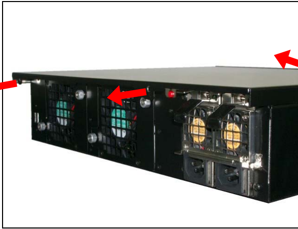
Fig. 2-3 Screws out from cover
