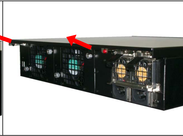
Fig. 2-4 Slide the cover backwards and pull the rear edge upwards
