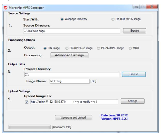
A very handy feature of the utility is point 4, which may be used to automatically upload the image to the board after a successful convertion. Enter the IP of your board and leave the other fields at defaults. Press the
