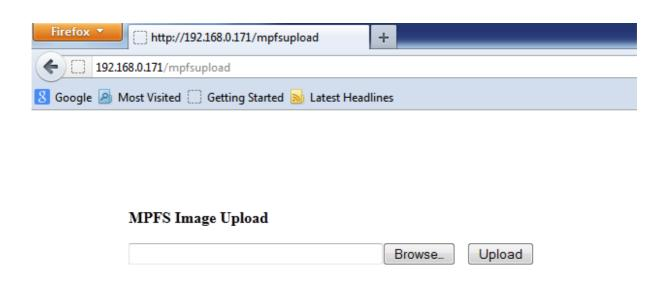
Click on the button "Browse\_" to select the "\*.bin" file you are about to upload. Select the image file in directory "PIC-WEB 5.42\TCPIP\Webpage MPFSImg prebuilt.bin" and press 'Upload'. Sit back and relax while the upload takes place and then navigate to the home page to behold the page just uploaded.
