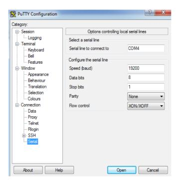
NOTE: The field "Serial line to connect to" should be with value depending on the com port where you have connected the board. You can check that on the device manager menu, category "Ports (COM & LPT)".
