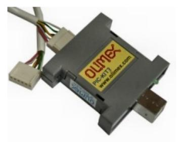
There are several ways to program a PIC, but the easiest and proper way to program the PIC-WEB is using a compatible programmer with an ISCP connector and compatible with MPLAB IDE. For this purpose it will be used an USB programmer compatible with MPLAB 8.87 and MPLABX 1.41 PIC-Kit3 sold by Olimex.
