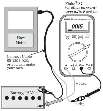
A good quality, adjustable, regulated DC power supply can be substituted for the 12-volt battery. The power supply should have at least 3 Amperes output, preferably more, and capable of overcurrent surges.
