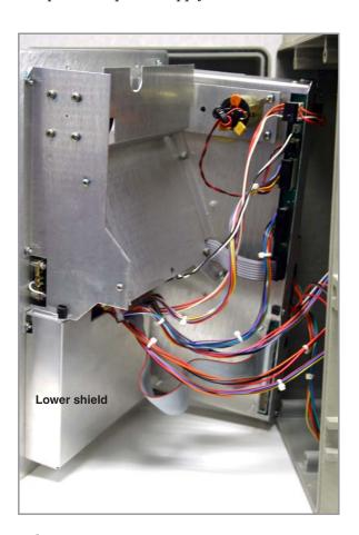
Figure 4-3 Flow meter with front panel removed
