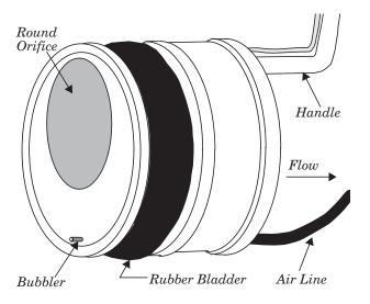
Figure 3-6 Flow Metering Insert
