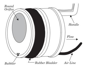
Figure 2-2 Flow Metering Insert
