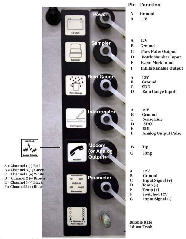
Figure 1-1 4230 Side View Showing Connectors and Pin Functions
