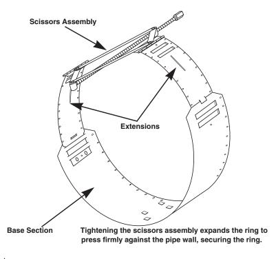
Figure 4-13 Scissors Ring Adjustment
