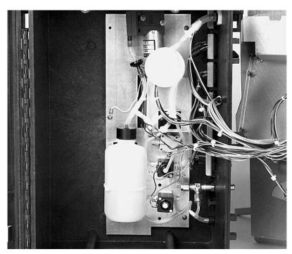
Figure 5-6 4230 Bubbler System Pressure Control
