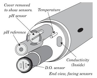
Figure 4-14 YSI 600 Multiple Sensor Sonde
