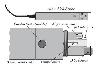
Figure 2-1 The YSI 600 Sonde
