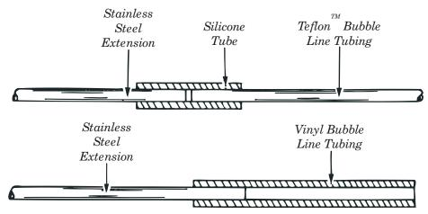
Figure 3-5 Installing the Stainless Steel Bubble Line Extension
