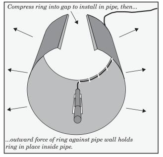
Figure 4-12 Sensor Installed on a Spring Ring
