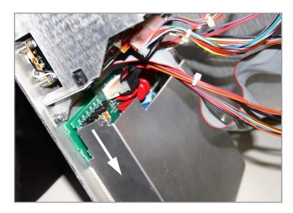
Figure 4-4 Removing the lower shield
