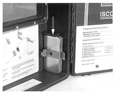
Figure 5-1 Location of the Case Desiccating Canister
