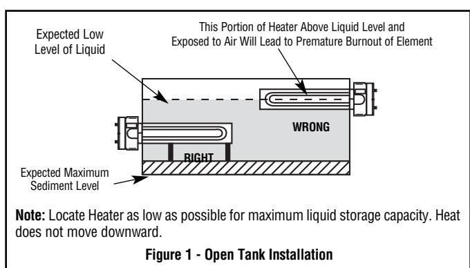
**Note:** Locate Heater as low as possible for maximum liquid storage capacity. Heat does not move downward.
