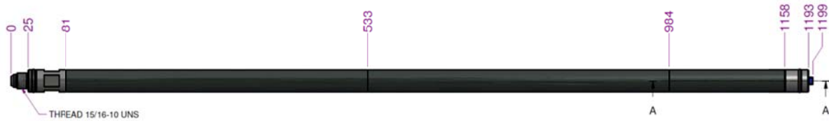
Figure 3.1 – The AD250 Downhole Gauge Important Dimensions
