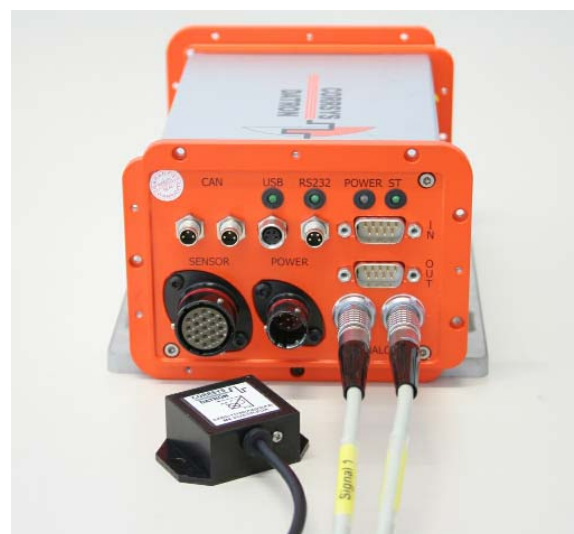
S-350 Sensor Electronics with connected Gyro
