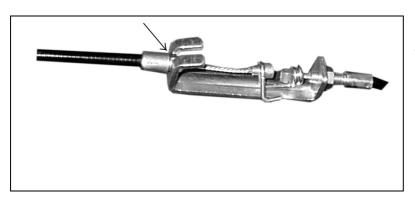
Drop down the Connector so the fitting sits firmly on top of the bracket.
