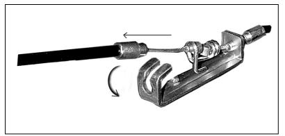
Pull the Upper Tension Connector backward and slide the wire through the slot on the bracket.
