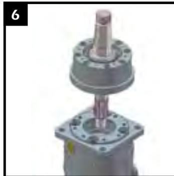
Lift up on the bearing box to remove from motor.
