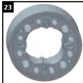
**STATOR:** Normal wear results in polishing of cam form which does not impair motor performances. Noticeable wear may be apparent along the corner of one side of the stator vane slot. This does not necessarily require replacement of the stator, but may slightly affect volumetric efficiency.
