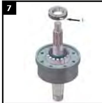
1) Loosen clamp screw in lock nut.
