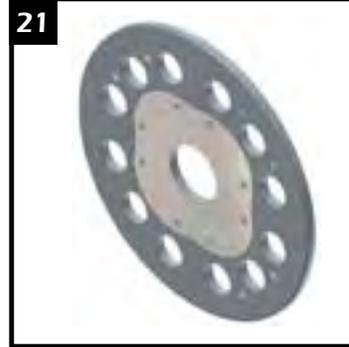
**PLATES:** Normal wear results in marking of timing plates which does not impair motor performance. Replacement of the timing plate is required if any smearing, galling, or heat cracks are present.
