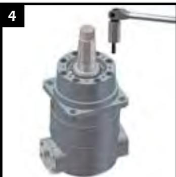
Loosen and remove 8 each 3/8" bolts with 5/16" socket head wrench.
