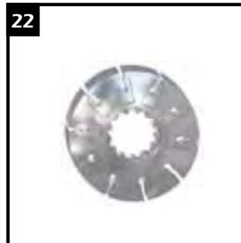
**ROTOR:** Normal wear results in polishing of rotor faces which does not impair motor performance. Examine the rotor vane slots closely. Polishing down in the slots is normal, but if there is any indication of a "pocket" forming in the wall of the slot, the rotor should be replaced.
