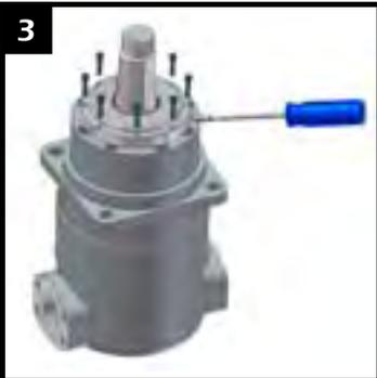
1) Loosen and remove 8 each 10-32 bolts.
