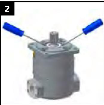
1) Pry out shaft seal plate with two screw drivers.
