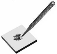
**1. Clean The Damaged Area**Use the Carbide tip probe carefully to probe the pit, freeing all the loose glass particles from the crushed cone, and to clean the hole of all the debris. Clear the loose glass from the break area. Clean the area surrounding the break with a dry cloth. Use glass cleaner if available.
