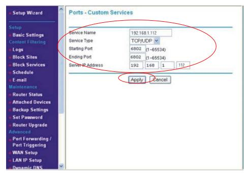
Type the IP in the **Server IP Address**, e.g. 192.168.1.112. Type the beginning port number in the **Starting Port** box. Type the same port number in the **Ending Port** box, e.g. 6802. \* Note: They must be the same as the data in DVR "Network Setting" menu.
