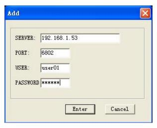
Type the IP/ domain name (e.g. 192.168.1.53 or dvrddns.kmip.net) and port (e.g. 6802) of the DVR which need added. Then type the network user's name (default user01) and the password (default 000000 or 111111) of the DVR. If the password is a super one, the playing speed of the video is faster. At last, click "Enter", the IP could be added.
