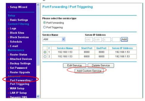
Click "Add Custom Service" in the figure above to pop up a new figure, you could set two groups of Service IP address and Port (Twice) as follows. One port is "80", the other one is "6802".
