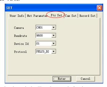
You could set baudrate, device ID and protocol of each camera.
