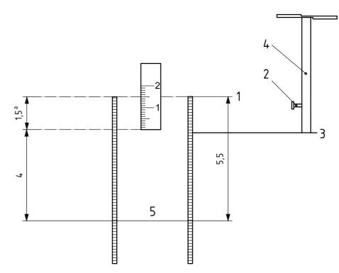
a) MP above LSD — Subtract MP correction to correct this water level to LSD (5,50 – 1,50 = 4,0)
