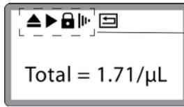
Display a status of the functions such as Eject, Start, Lock or Insert. (status of slide holder)
