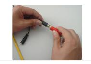
(3) Insert the output plug of 12V adapter into the power input connector of microscope
