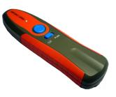
The universal connector can be used for all the most widespread fiber interfaces such as ST / SC / FC connector. It is suitable to test both Singlemode and Multimode cables. With an optional 2.5 mm to 1.25 mm optional Adapter, you can easily test 1.25 mm diameter fiber LC or MU connector. The visibility is up to 3 Km to 5 km depends upon the output power of the Fiber Checker.
