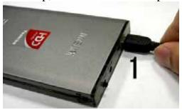
Second step, connect the additional USB cable to USB1 port on Movie Spot
