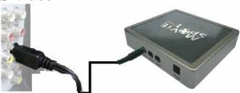
You must locate the Video cable supplied with your Movie-Spot. On one end of the Video cable are a thick black plug and a yellow plug. On the other end of the Video cable is a skinny black plug. Connect the skinny black plug of the Video
