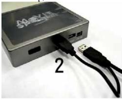
Final step, wait for 3 seconds, then connect the other USB cable to USB2 port on Movie
