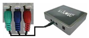
The Component Video cable can be purchased to obtain the highest quality video. On one end of the Component Video cable are three plugs, colored red, green, and blue. On the other end of the Component Video cable is a single skinny black plug.
