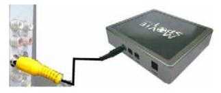
You must locate the Video cable supplied with your Movie-Spot. On one end of the Video cable are a thick black plug and a yellow plug. On the other end of the Video cable is a skinny black plug. Connect the skinny black plug of the Video cable into the Video port on your
