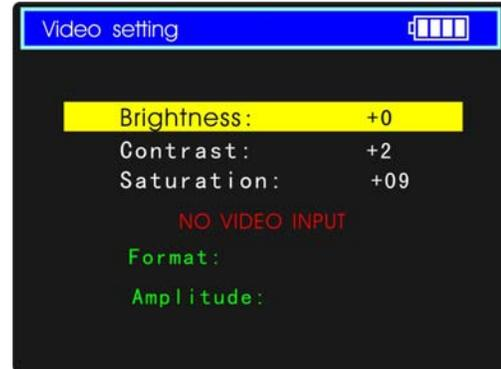
Depending on the type of camera connected to the ST-F35TEST, the Video “Format” will automatically change between NTSC and PAL, and the Video Level will automatically change between IRE (Institute of Radio Engineers) and mV. NTSC signals measured in IRE units, PAL signals measured in mV.
