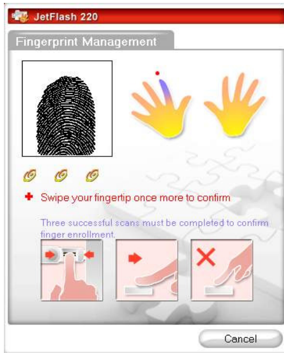
Figure 8. Three successful scans must be completed to confirm finger enrollment
