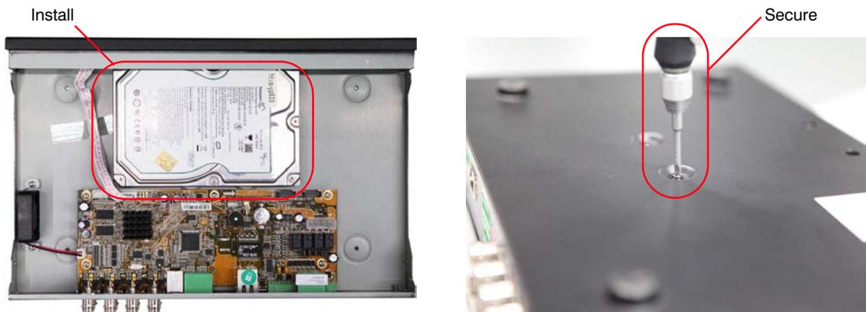
3. Remove the HDD data line from the accessories box. Plug one end of the data line to the circuit board, and the other end to the data line port on the HDD. Connect the power cord to the HDD in the same way.
