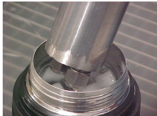
Figure 21 Stack Thermocouple in Ice Bath
