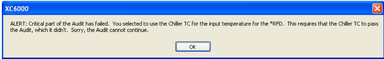
Figure 27 Chiller Thermocouple Sensor Test FAILED
