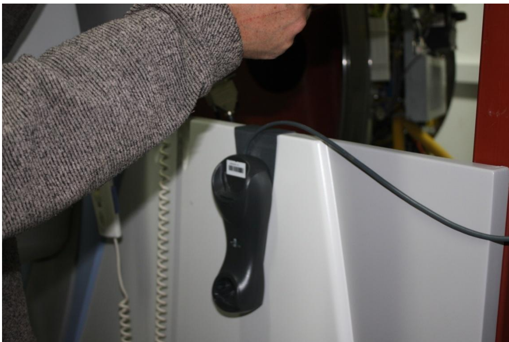
Figure 9: Cradle for the bar code scanner attached to the cradle bracket
