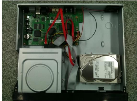
6. A picture after installation of the HDD.
