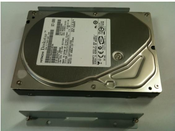
1. Before installing the HDD bracket and screws.
