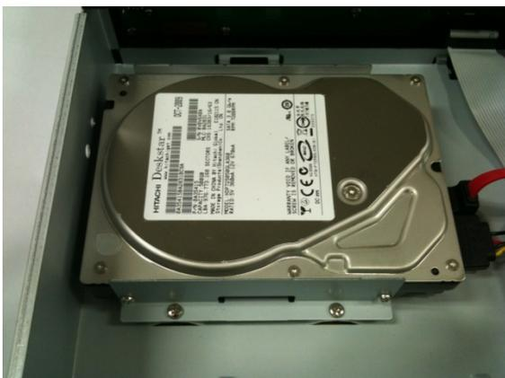
3. Install the HDD and Bracket onto the base of the case (inside).
