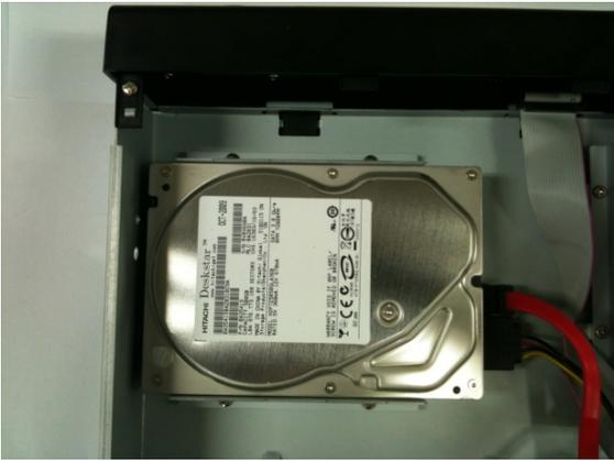
5. After connecting the power and data cables to the HDD.
