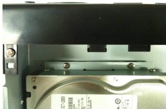
4. Install the HDD and Bracket onto the base of the case (outside).
