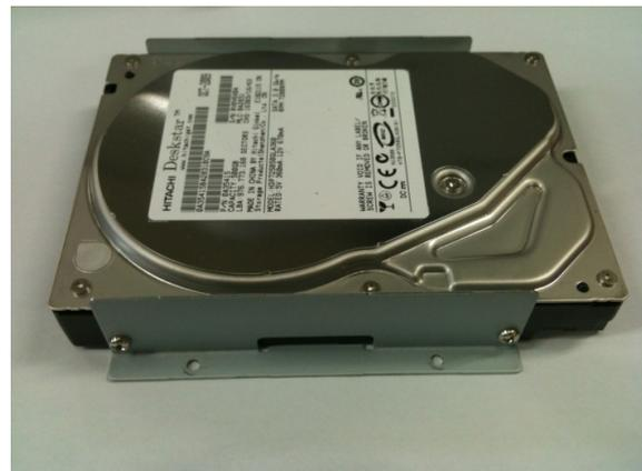
2. After installing the HDD bracket and screws.
