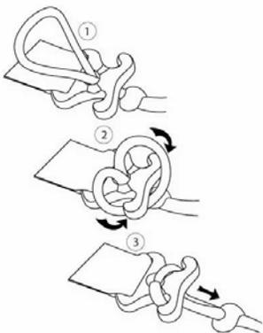
Attach a properly rated tow rope (not included). **Important:** Loop end of rope **MUST** pass through hole of the quick-connect prior to wrapping loop around hooks. Inspect condition of molded tow point prior to each use. Do not use if it shows signs of damage, cracking or breaking.
