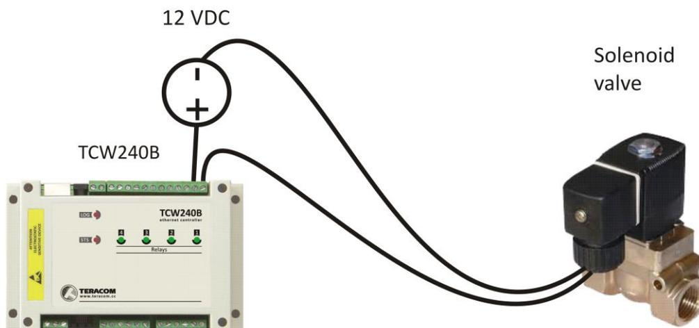
For loads with higher switchable current/voltage than specified, an external relay should be used.
