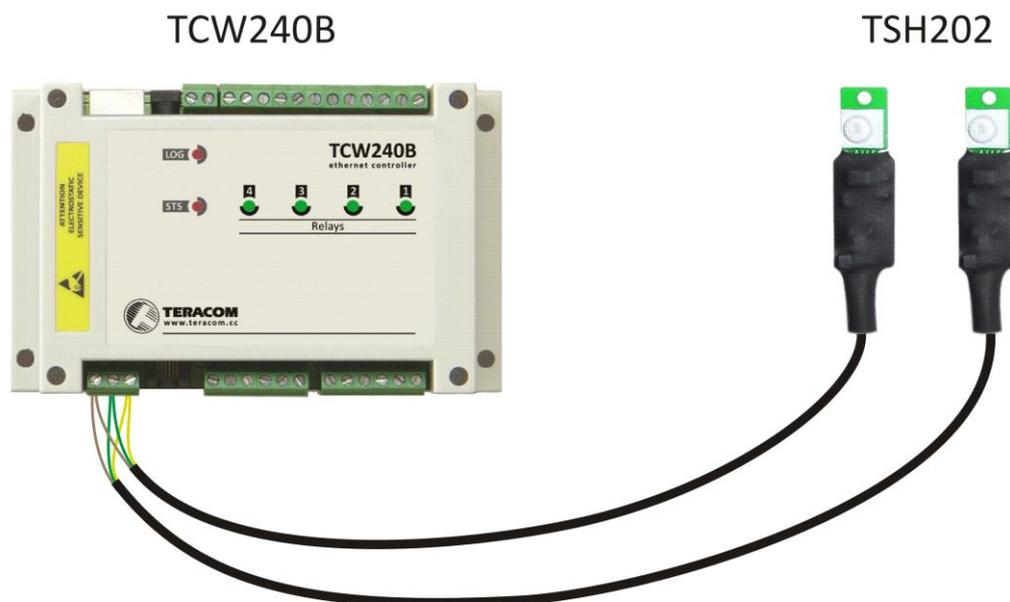
Connections can be realized either by screw terminal connector or by standard RJ-11 connector.
