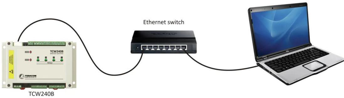
For configuration, **TCW240B** may be connected directly to the Ethernet port on a computer. The device support Auto-MDIX and it is not necessary to use “crossover” cable, standard “straight-through” can be also used.
