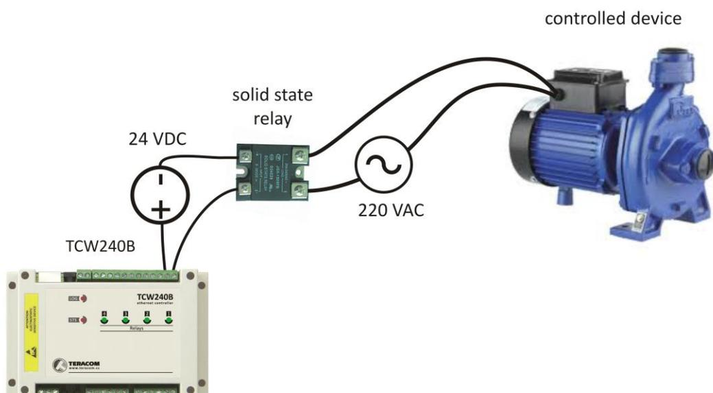
When mechanical relays switch inductive loads such as motors, transformers, relays, etc., the current will arc across the relay contacts each time the contacts open. Over time, this cause wears on the relay contacts which shorten their life. When switching an inductive load, it is recommended that relay contact protection devices are used.
