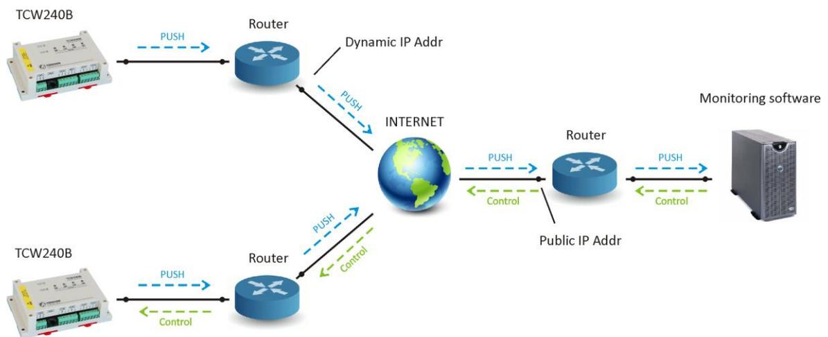
The main advantage of the PUSH technique is that the controllers can be installed in private networks (behind the routers without port forwarding arrangement). The server should have public IP address.
