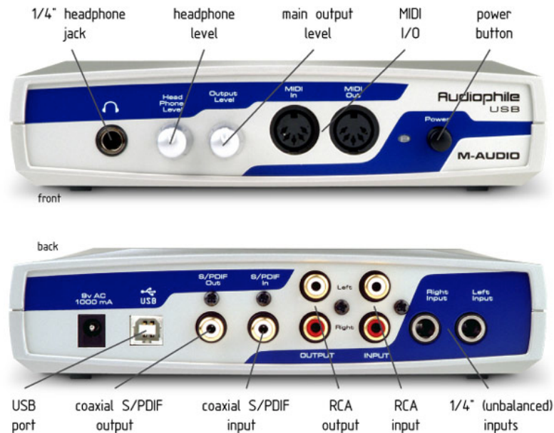
figure A.3 - M-Audio Audiophile USB device front and back view
