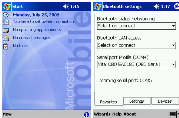
Figure 18 – Pocket PC Desktop with a Bluetooth Add-on (not built in). The Bluetooth Icon is shown in the Bottom Right Corner. The Serial Port shown here is COM4.
