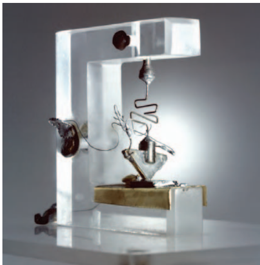
"The first transistor ever assembled, invented in Bell Labs in 1947." Photo and text from Porticus.org, www.porticus.org/bell/belllabs_transistor.html . (Follow that link to see more historical documents and images about Bell Labs and the transistor.)
