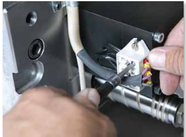
Figure 11-14 Removal of wires from wire harness
