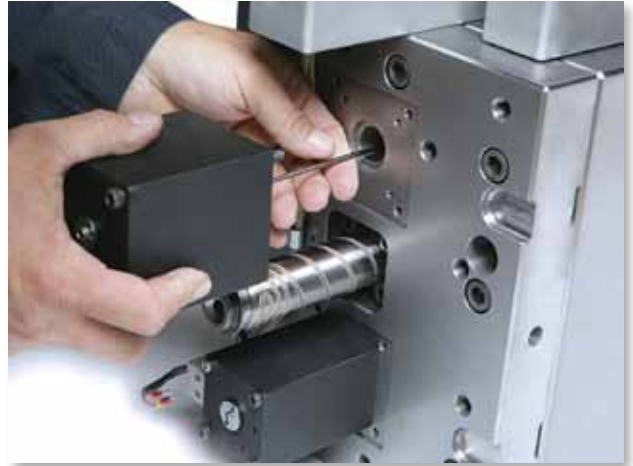
Figure 11-16 Removal of unit from hot half
