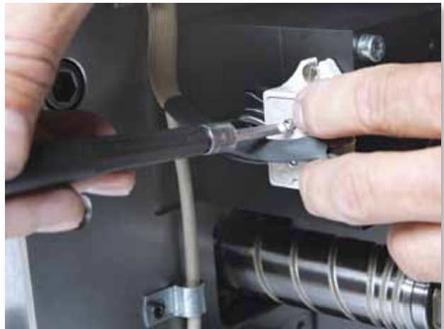
Figure 11-21 Install wiring cover plate
