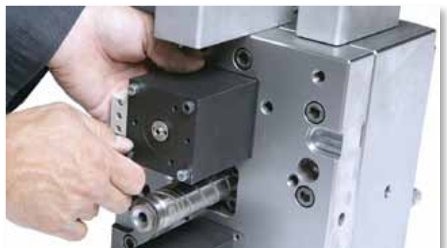
Figure 11-18 Insert E-VG mounting screws
