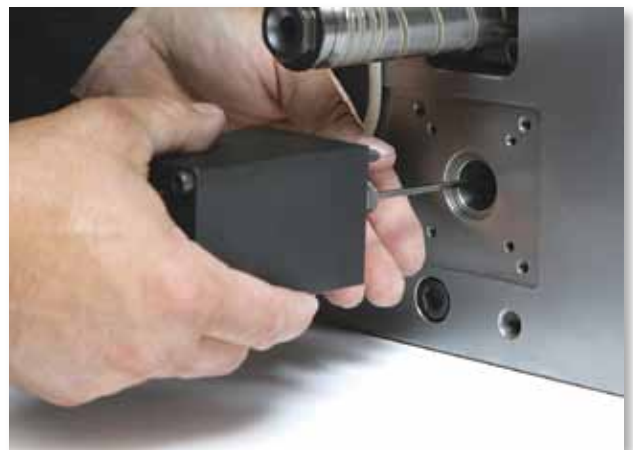
Figure 11-17 Insert valve pin into valve bushing
