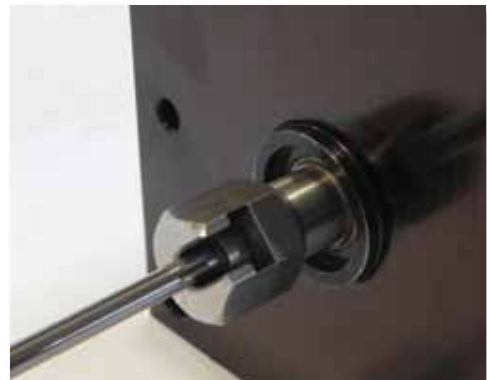
Figure 11-8b Pin in Pin Holder T-Slot
