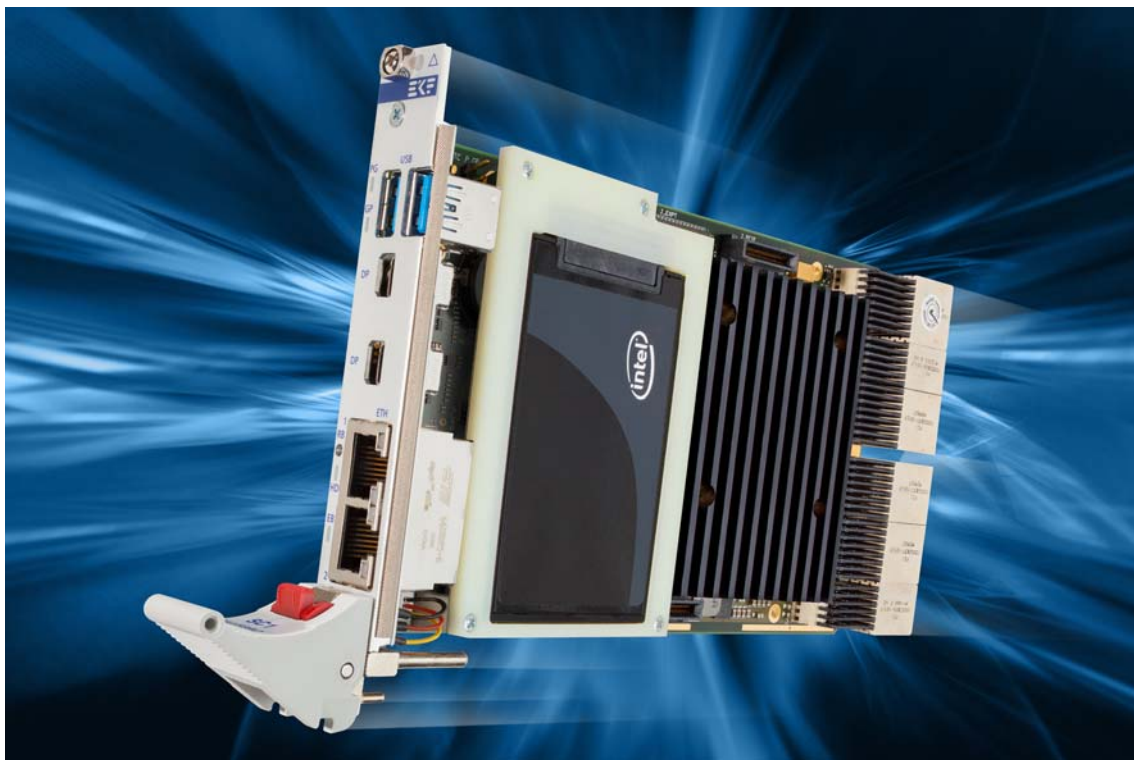
4HP Front Panel Width with C42-SATA
