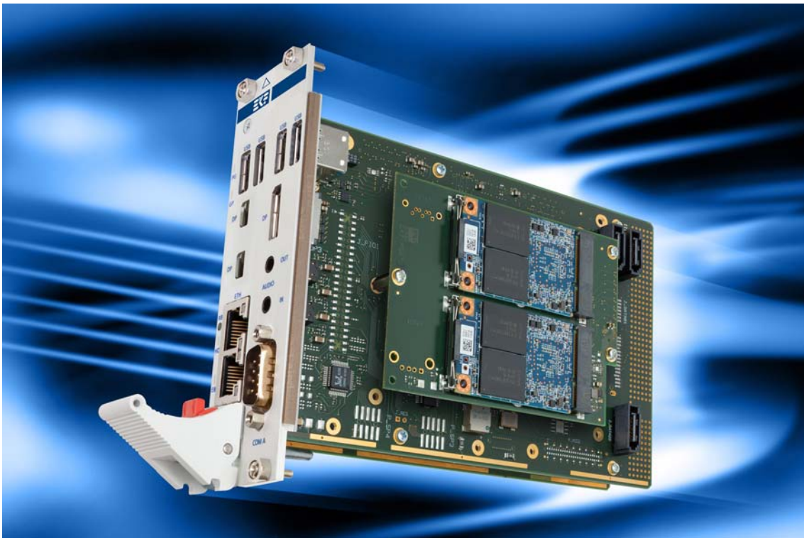
8HP Assembly w. PCS-BALLET Side Card & C47-MSATA
