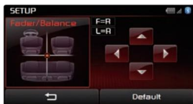
2. Use the **▲**, **▼**, **◀**, **▶** buttons to make adjustments to the sound position.
