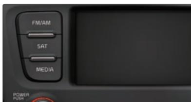
1. Press the **FM/AM** key on the control panel. The most recently played FM/AM radio band will automatically begin playing.
