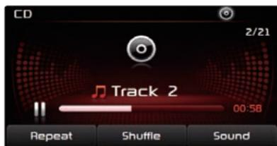
2. When a track is playing and you wish to pause, press the **||** button next to the progress bar. Press the **▶** button to restart the track.
