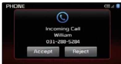
1. Press the **Reject** button on the screen or the
