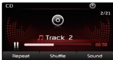
Press the **Sound** button on the main screen of each audio mode (FM/AM, SIRIUS, MEDIA, JUKEBOX) to enter Sound Setup.
