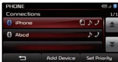
5. Once pairing is complete, the handset device will be shown in the Connections list.
