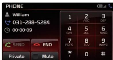
3. Press the **SEND** button on the screen or the **SEND** key on the steering wheel controller to connect the call.
