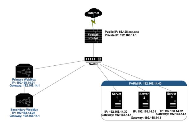
In Single Network Mode, connections being load balanced and going to the real servers will appear to come from the WebMux itself. You will not need to make any changes on your servers since the servers will always reply back to the WebMux when sending back their reply. You will only need to connect the "server LAN" side of the WebMux to the network.
