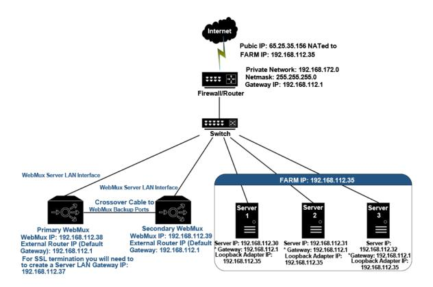
The above diagram is an example about how to configure the WebMux in Out-of-Path Mode without changing the IP addresses of the web servers and other servers that already exist on the network. This is another option that can be used if changing the existing network topology of the servers causes problems.
