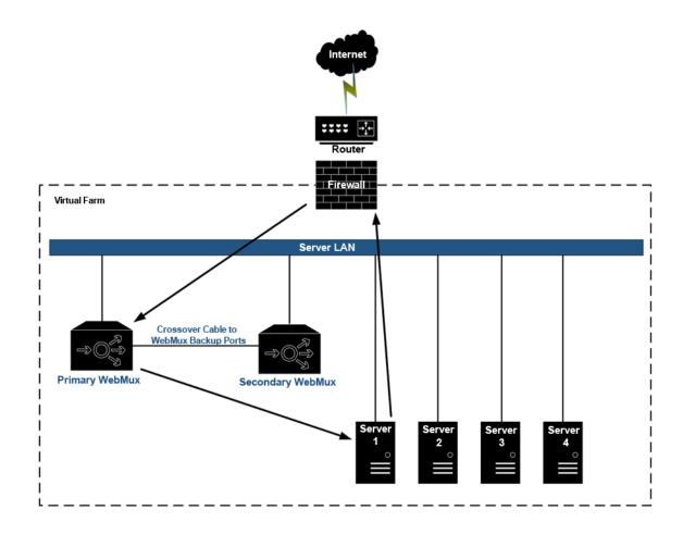
In most situations, incoming traffic is in small requests and return traffic from servers back to clients is large amounts of data (pictures or documents). Using Out-of-Path Mode will allow up to 100 times more traffic to be handled by the WebMux load balancer. The disadvantage for OOP/direct response is that the firewall protections built in to the WebMux will no longer function. Users must provide their own firewall for incoming and outgoing traffic.
