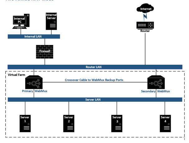
The main purpose of the WebMux is to balance IP traffic amongst multiple web or other servers. The diagram above shows a NAT installation with two WebMux units. In this configuration, one WebMux is serving as the primary, and the other is serving as the secondary, or backup, providing a fault tolerant solution.
