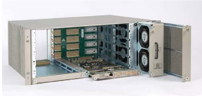
Figure 21 – Extracting a Fan Tray
