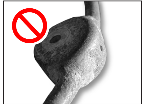
An Anode Ring with pronounced oxide coating.
