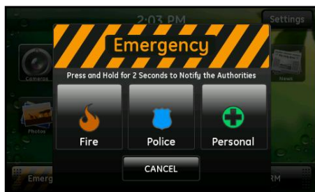
Figure 9. Fire, Police, and Personal emergency buttons
