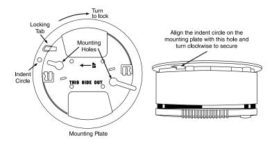
Locate the smoke detector mounting plate on the wall or ceiling and mark all desired screw locations. Use the supplied wall anchors for all screw locations. When the anchors have been placed, secure the mounting plate to the ceiling or wall.
