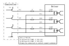
Figure 4: Connection to PNP signal (common-cathode)
