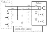
Figure 3: Connections to open-collector signal (common-anode)
