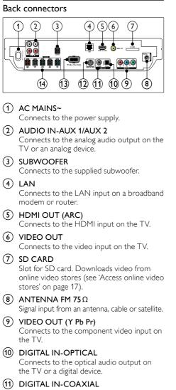
Connects to the coaxial audio output on the TV or a digital device.
